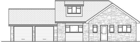
Proposed South Elevation 1:100
