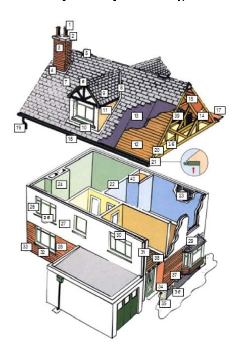
2 Coping stone 3 Chimney head Flashing 4 Ridge ventilation 5 Ridge board Slates/tiles 8 Valley guttering 9 Dormer projection Dormer flashing 10 Dormer cheeks 11 12 Sarking Roof felt 13 Trusses 14 15 Collar 16 Insulation 17 Parapet gutter Eaves guttering 18 Rainwater downpipe 19 20 Verge boards / skews 21 Soffit boards 22 Partition wall Lath / plaster 23 24 Chimney breast 25 Window pointing Window sills 26 27 Rendering Brickwork / pointing 28 Bay window
