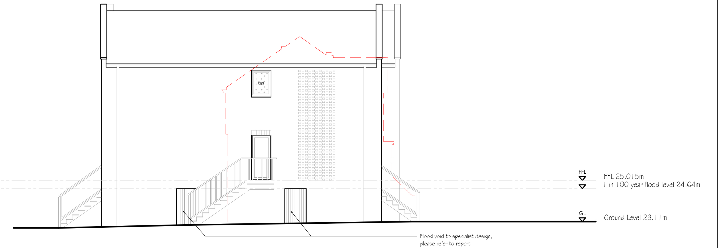
Proposed Side (North) Elevation 1:100
