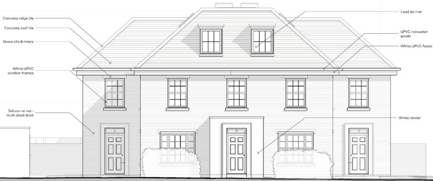
West Elevation - As Proposed 1: 50
