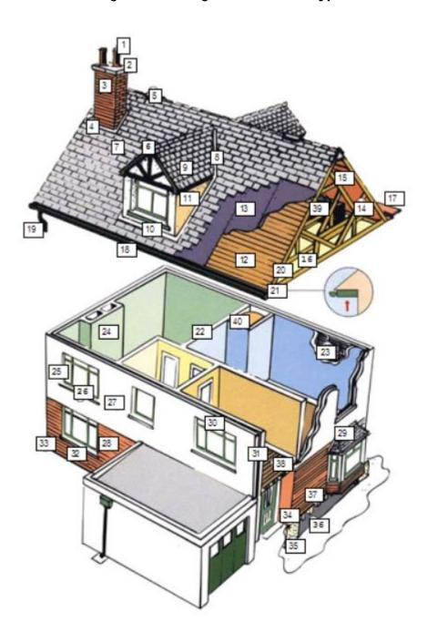
Coping stone 2 3 Chimney head Flashing 4 Ridge ventilation 5 Ridge board Slates/tiles 8 Valley guttering 9 Dormer projection Dormer flashing 10 Dormer cheeks 11 12 Sarking Roof felt 13 Trusses 14 15 Collar 16 Insulation 17 Parapet gutter Eaves guttering 18 Rainwater downpipe 19 20 Verge boards / skews 21 Soffit boards 22 Partition wall Lath / plaster 23 24 Chimney breast 25 Window pointing Window sills 26 27 Rendering Brickwork / pointing 28 Bay window 29 30 Lintels
