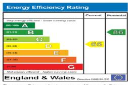
The energy efficiency rating is a measure of the overall efficiency of a home. The higher the rating the more energy efficient the home is and the lower the fuel bills will be.
