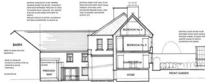
WEST ELEVATION (COURTYARD)
