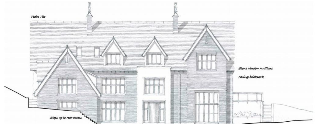
Front Elevation facing North West
