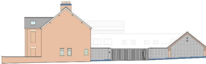
NEW TIMBER/COMPOSITE SLIDING GATES AND WALL TAKEN UP TO 1.8M
