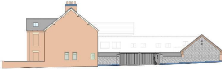
EXISTING WALL HEIGHT WITH SHALLOW TIMBER/COMPOSITE PANELS; EITHER FIXED OR HINGED INTERNALLY TO FOLD BACK-TO-WALL FOR INCREASED NATURAL LIGHT AND/OR VIEWS AS REQUIRED
