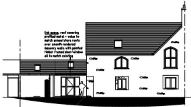
west elevation yard wall omitted for clarity
