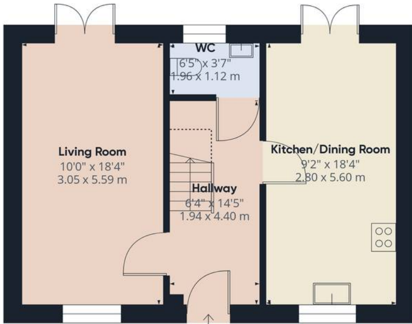
Ground Floor Building 1
