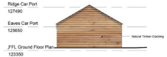
Item No. 10 Name - Proposed West Elevation Car Port Scale - 1:100
