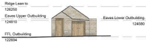
Item No. 9 Name - Proposed West Elevation Outbuilding 1 Scale - 1:100
