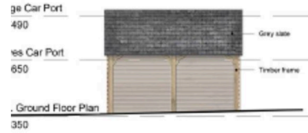
Item No. 7 Name - Proposed North Elevation Car Port Scale - 1:100
