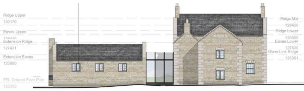
Item No. 2 Name - Proposed North Elevation Scale - 1:100
