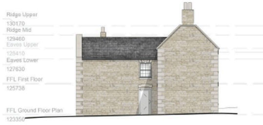
Item No. 5 Name - Proposed West Elevation Scale - 1:100
