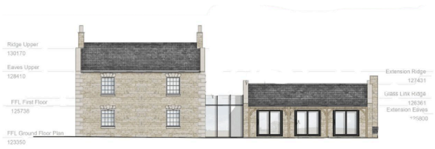
Item No. 4 Name - Proposed South Elevation Scale - 1:100
