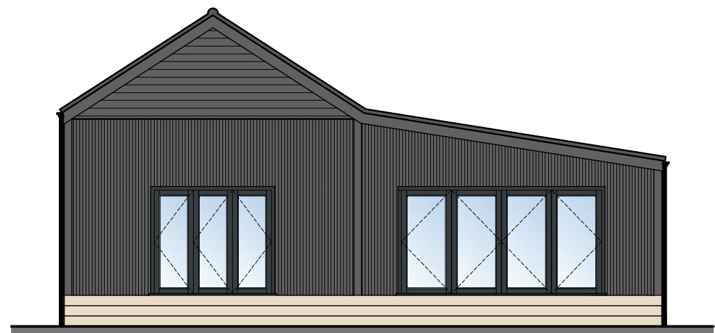
PROPOSED REAR ELEVATION (south) SCALE: 1:100
