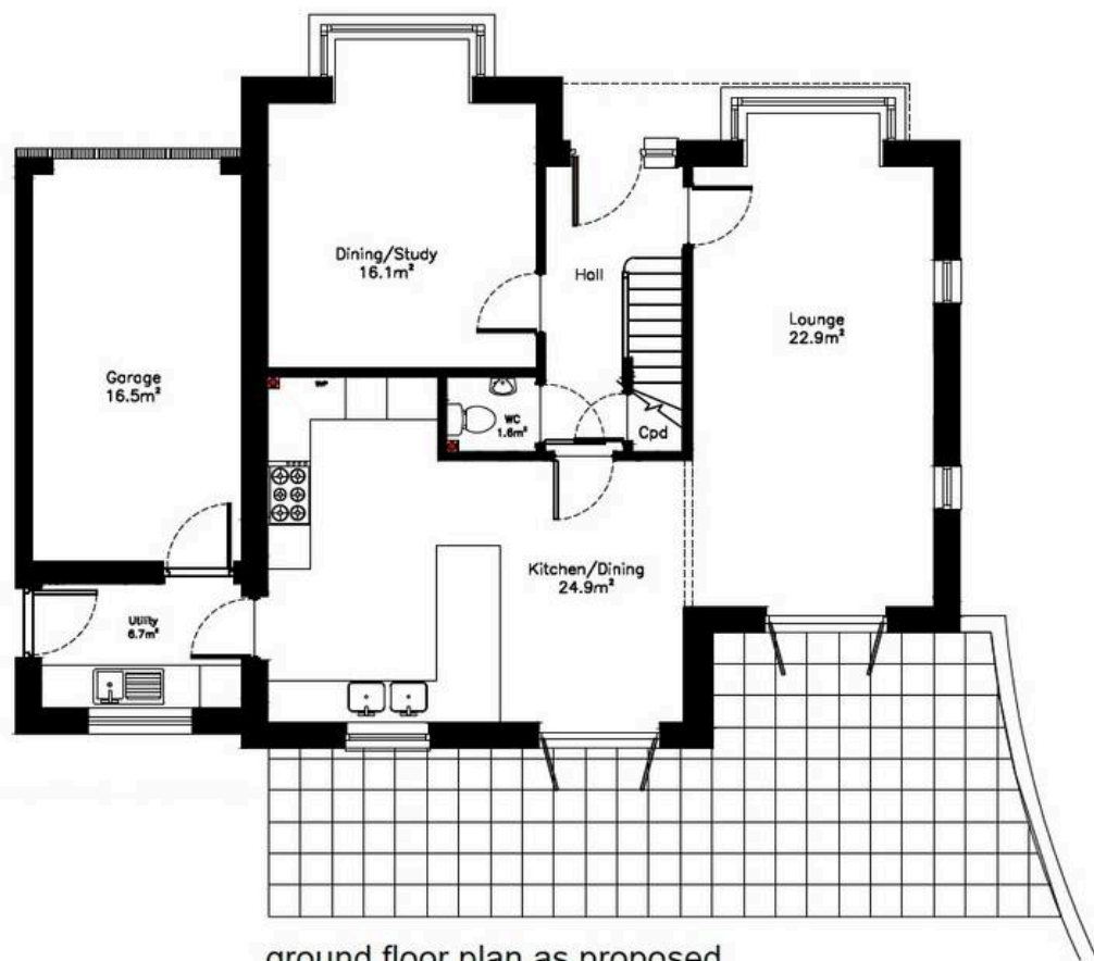
ground floor plan as proposed floor area = 81.2m 2 excluding garage
