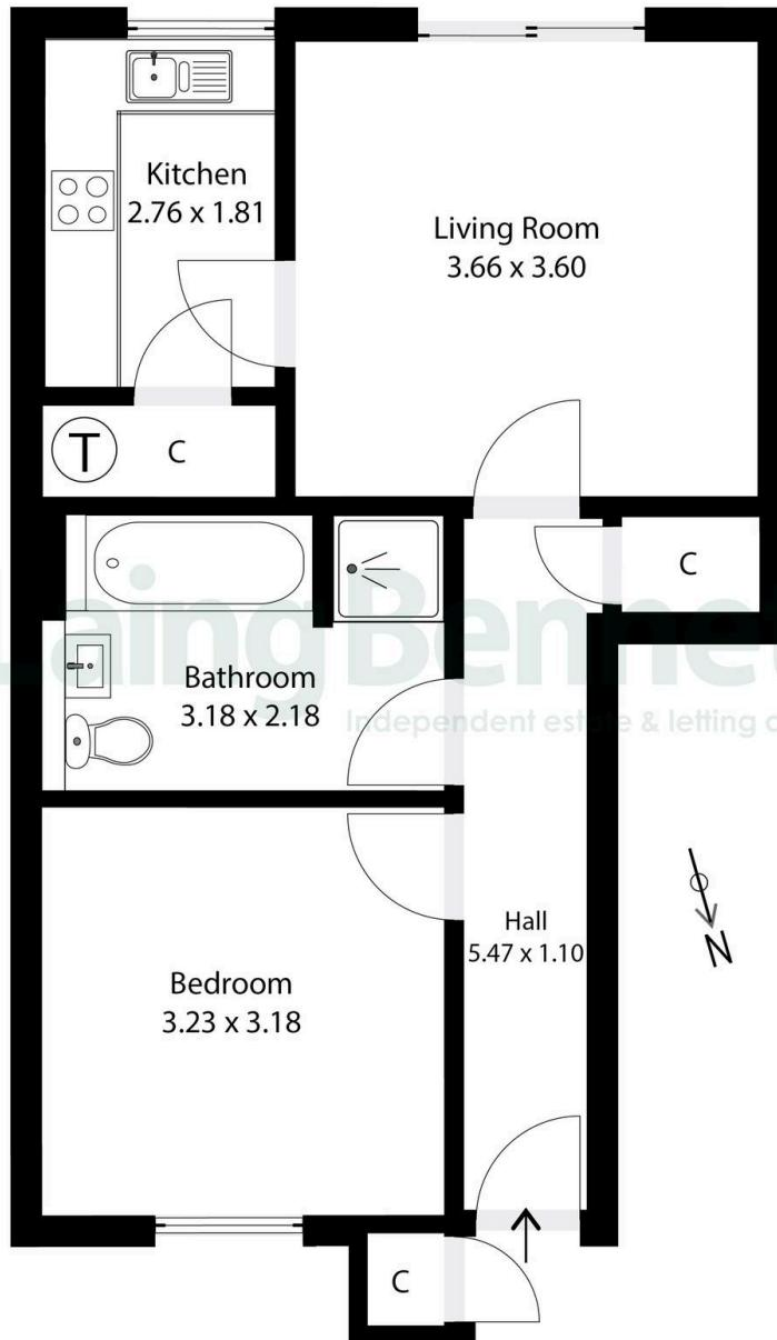
Illustration for identification purposes only. Measurements are approximate. Dimensions given are between the widest points.
