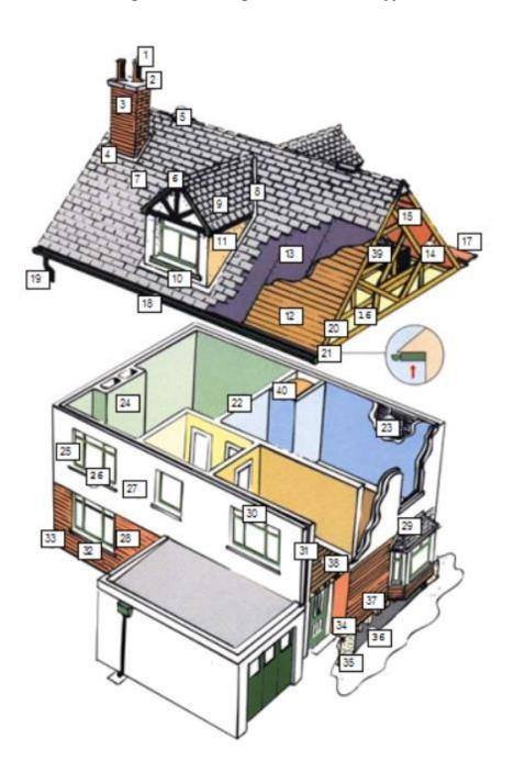
3 Chimney head 4 Flashing 5 Ridge ventilation 6 Ridge board Slates/tiles 8 Valley guttering 9 Dormer projection 10 Dormer flashing 11 Dormer cheeks 12 Sarking 13 Roof felt 14 Trusses 15 Collar 16 Insulation 17 Parapet gutter 18 Eaves guttering 19 Rainwater downpipe 20 Verge boards / skews 21 Soffit boards 22 Partition wall 23 Lath / plaster Chimney breast 25 Window pointing 26 Window sills 27 Rendering 28 Brickwork / pointing
