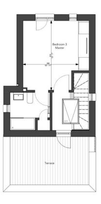
Automatic opening smoke vent (AOV) at head of stairs linked to fire detection in stair core. THREE BEDROOM
